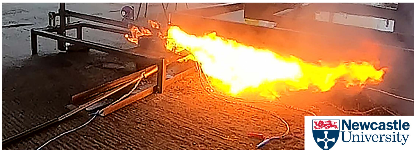
Figure 3: Flare-like flame, approximately 3 metres long, resulting from nail penetration of a lithium-ion battery electric vehicle module
